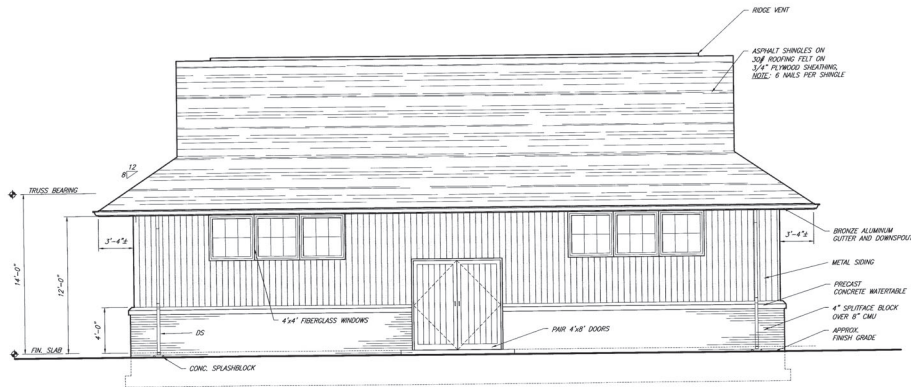
SOUTH ELEVATION (NORTH ELEVATION SIM.) 1/4\" = 1'-0"
